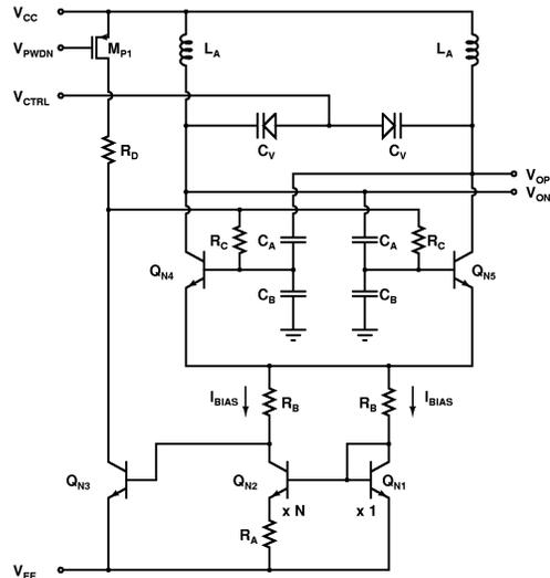
Fig. 1. VCO schematic (VCO embedded in Widlar-bandgap).
