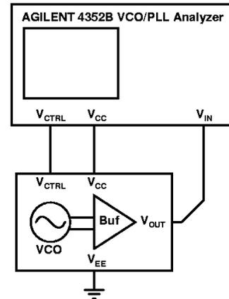
Fig. 5. Measurement setup.
