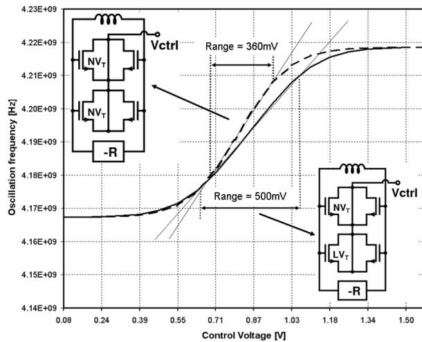
Fig. 7. Simulated range extension for a VCO circuit [13].
