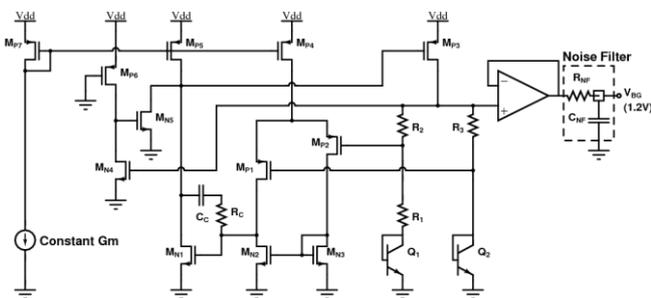
Fig. 5. A simplified band-gap circuit with noise filter.
