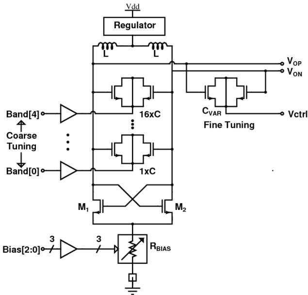
Fig. 2. A conceptual NMOS VCO circuit diagram
